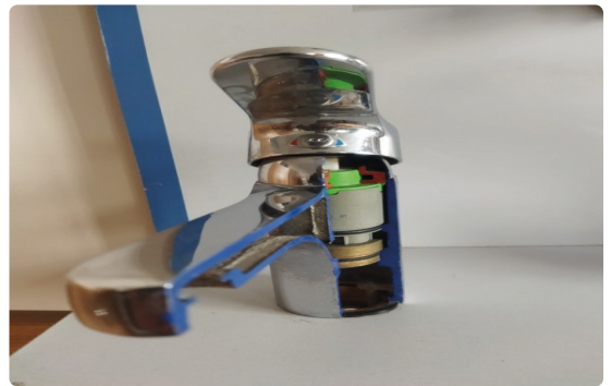
Görsel 11.5: Batarya kartuşlu salmastra kesiti
