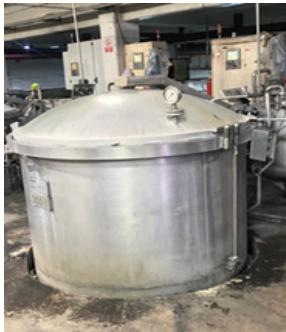
Görsel 6.2: HT elyaf-bobin boyama makinesi
