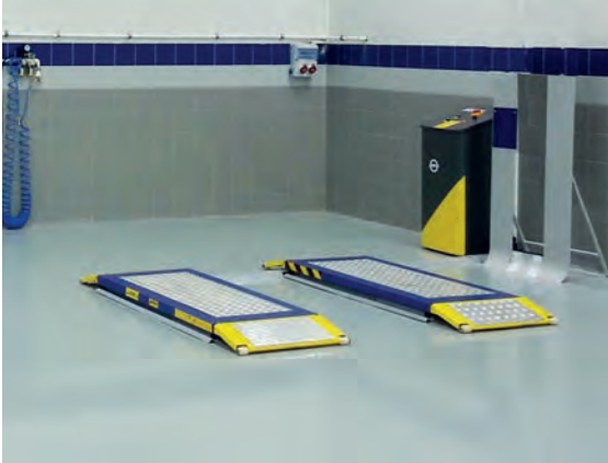
Görsel 3.107: Zemine monte makas lift
