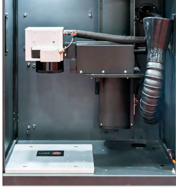
Görsel 6.4: CNC lazer markalama makinesi (galvo lazer)
