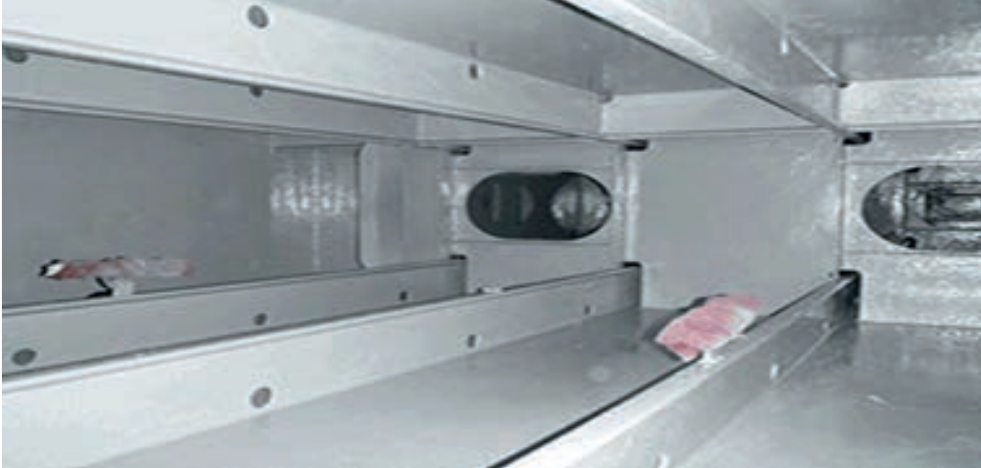
Görsel 8.34: Balast tank
